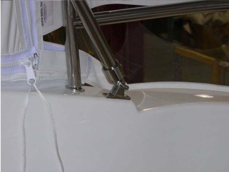
3. Bend the track at the back of the arch and in front of the rail stanchion so any water will be shed over board. Repeat on the opposite side.
