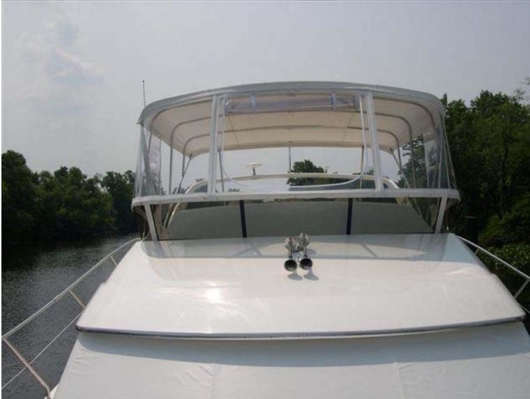
5. Begin with the front curtains. The buttons have not been installed in the panels to allow for adjustment on each boat. Use reference marks on each curtain to locate the windshield clips on the frame. Working from the center out to each side mark and install buttons one at a time.
