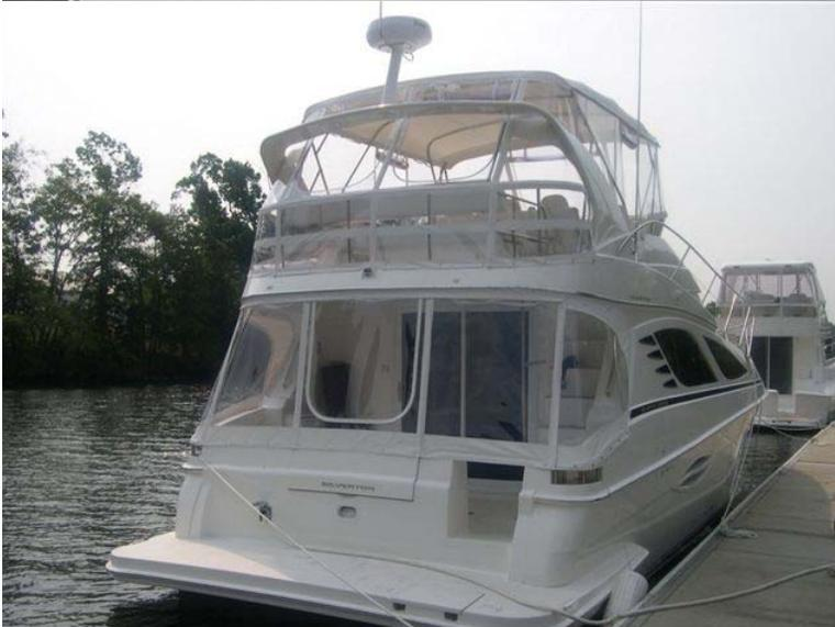
6. Install back curtains by lining the center zipper with the anchor light. Work out to each side installing the lift the dot studs provided.
