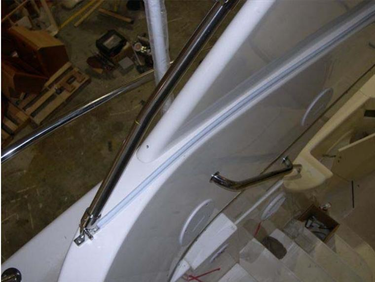
2. Track for the enclosure is packed with the frame. Install the flex track inside the arch as shown in this picture. Start outside the main and work to the back so that the track follows the inside edge of the bridge. Install the flex rail screws provided about every 4in.
