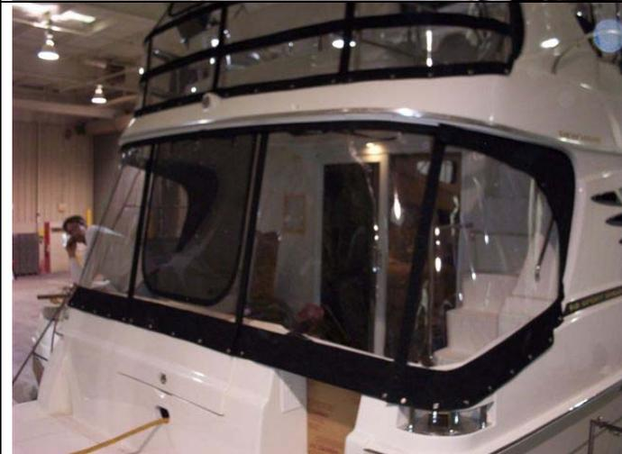
8) Start installing the center panel aligning the zippers with the transom hatch. Work outboard marking 1 or 2 buttons at a time, keeping the panels tight and smooth. Calk all holes and install all LTD studs provided.
