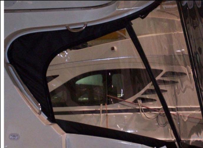
7) The side panels have a sheyed valance as shown in this picture. Slide the valance into the track and then zip the panel in place.
