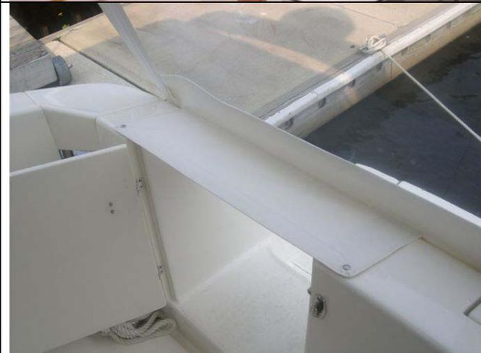
9) The last step is to install the door flap. Use the GB studs provided.
