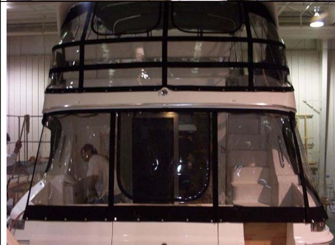
6) The back 3 panels have a valance that slides into the track. Once the valance is in place zip the panels on and to each other. The door panel has a flap to cover the opening left by the door.
